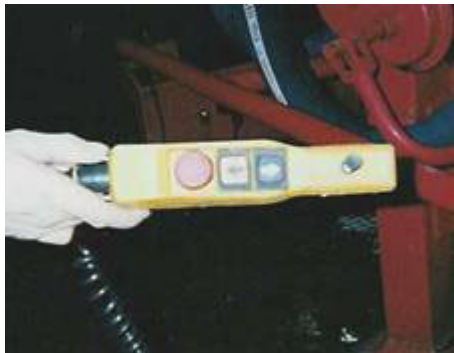
Controls for electrical tipping system
