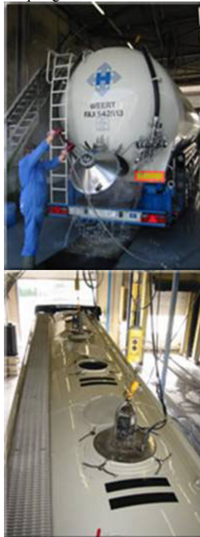
Above you can see a typical tanker cleaning installation.
