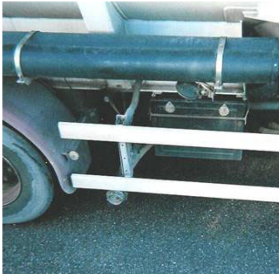
An example of the air control valves being situated on the side of the vehicle.
